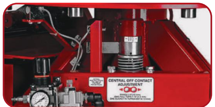
Mechanical central off-contact adjustment
