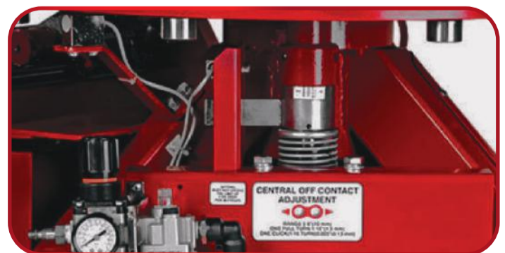
Mechanical central off-contact adjustment
